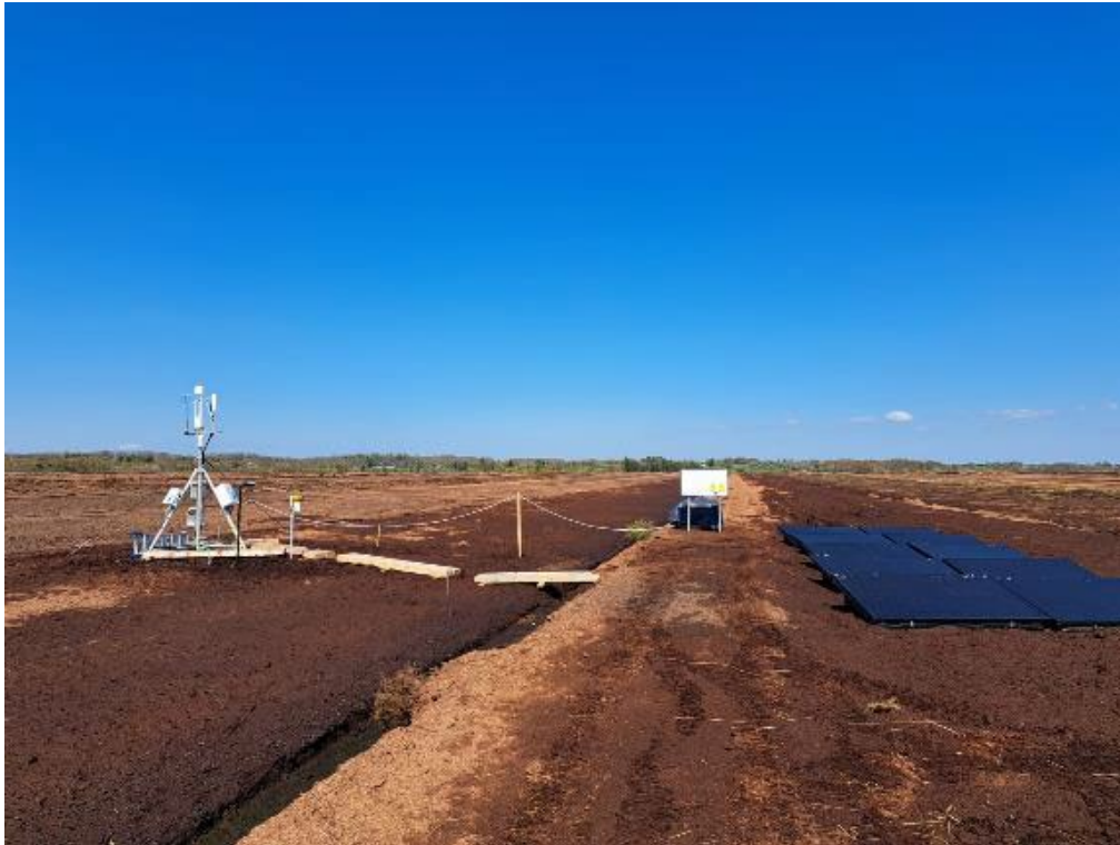
Figure 4.8: Flux tower tower in operation at site 2 location was selected because of the presence of deep peat, location away from stockpiles and presence of a significant footprint.
