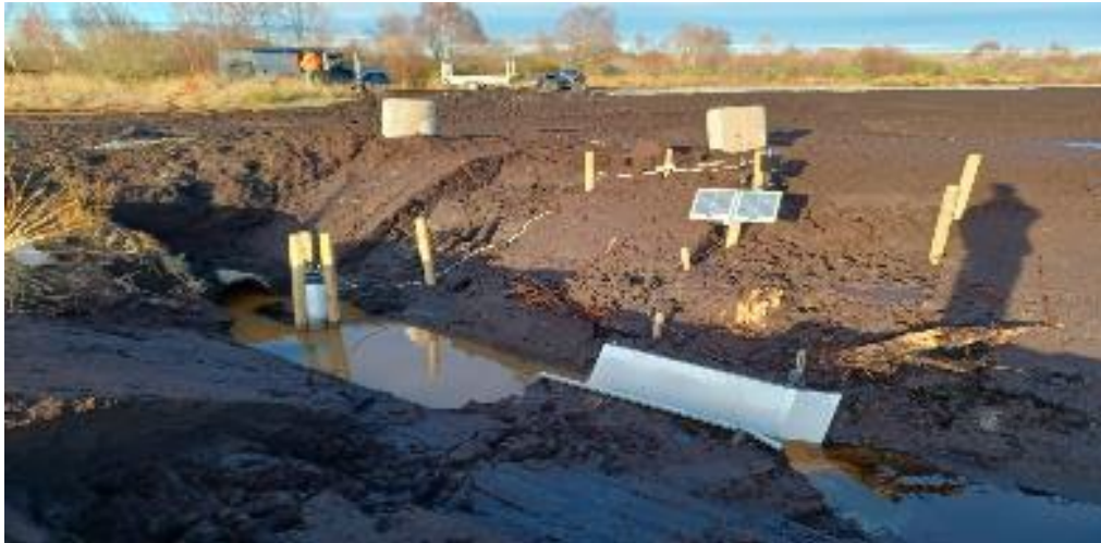
Figure 4.9: RBC Flume located in bare peat catchment of 42 hectares.
