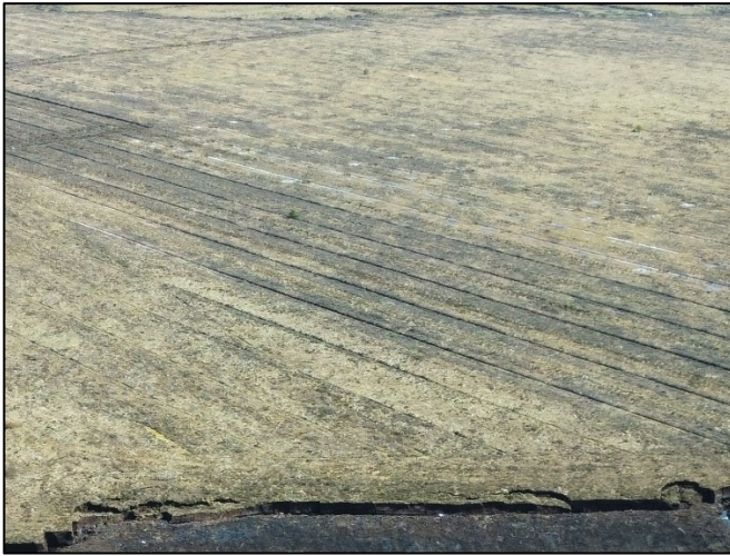
Plate 3-3 Drone image showing cutover bog (foreground, open drainage ditched (middle ground) and previously blocked drains (background).
